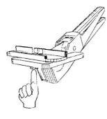
To change the guide fence position, make sure the blade is "pressed down" below the table top. Do not change the guide fence position with the blade open!! Push up the fence spring retainer button on the under-side of the table (see sketch below) and turn the fence until the alignmentpins align with the holes in the table.
