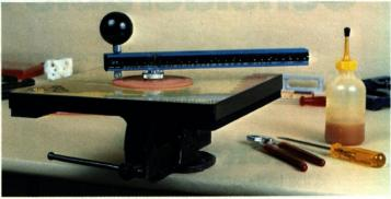
Place the gasket material on the cutting surface, set the cutting radius and rotate the cutter.
